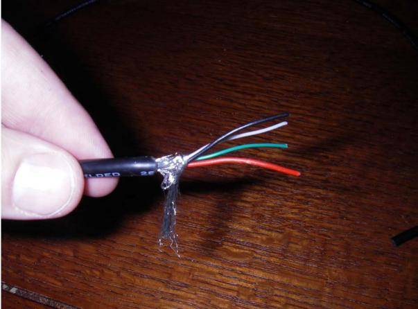
**Step 4:** The Zodiac AC charger cable contains a loose copper wire (- or ground) and a white wire (+). Strip ½ inch from the white insulated wire. Twist the free ends of the wires to neaten them up.
