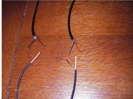
**Step 5:** Next take Zodiac connector cable and the male USB cable end. Twist together the white wire from the Zodiac cable with the red wire from the USB Cable.
