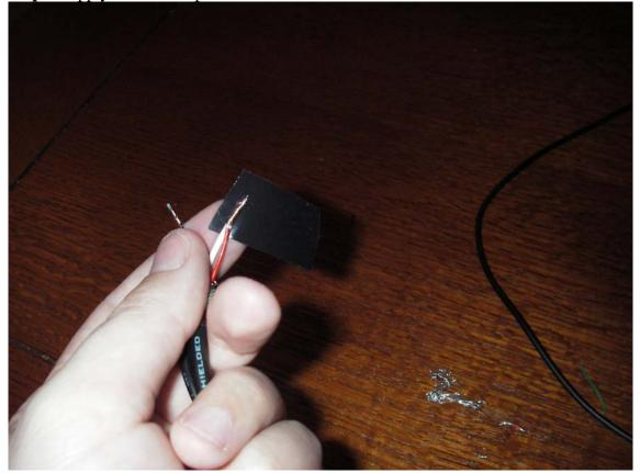
Step 7: Fold the taped wires over and tape over them and around the red and white wires,
