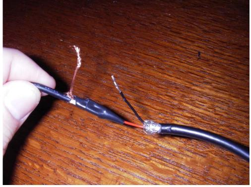
Step 8: Then twist the black wire and bare copper wire together (no point in taping since the other wire isn't
