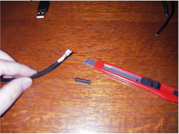
Step 3: The wires inside the USB cable will be surrounded by a wire mesh and metal foil shield, pull this apart to expose the 4 wire inside then clip off the wire mesh and foil to get it out of the way. Also cut away the green and white wire (you won't be using them). Next strip the insulation from ½ inch from the ends of the red and
