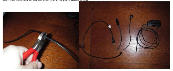
**Step 2:** Strip the outer layer of insulation from the two ends of the USB cables and from both ends of the Zodiac AC charge cables about 2 inches from the ends.
