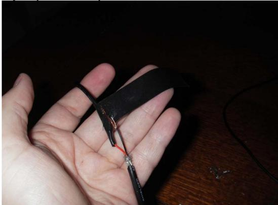
Step 10: To give the splice some strength, fold it over and back on itself and tape the two wire firmly together.
