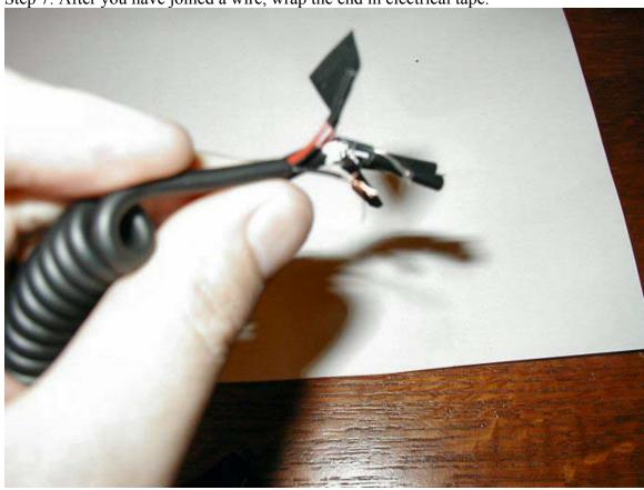
Step 8: Fold the taped end back along the wire length and then tape over both tape and wire again. (Do the same for both the red and black wires)
