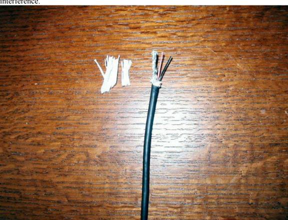
Step 3: Remove the wire mesh shield surrounding the USB cables. This exposes 4 little wires-- green and white for data, black for ground red for power (used for hotsync only, not connected to charger). Bend the tips and tape them over to prevent shorts (not sure if this would actually do anything but seems a prudent precaution).
