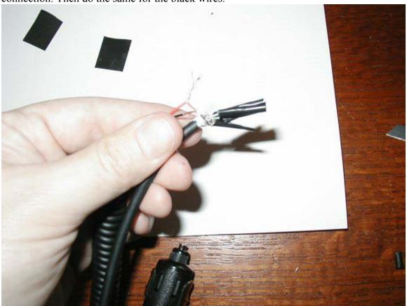
Step 7: After you have joined a wire, wrap the end in electrical tape.
