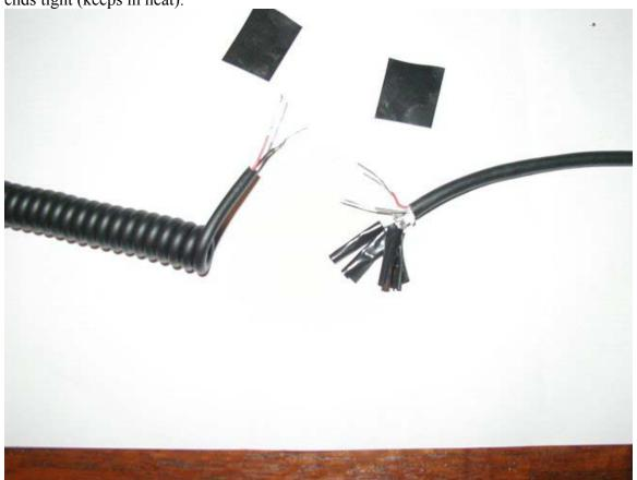
Step 6: Join the red wire from the car charger to the red wire from the adapter by twisting them together. You may want to add a drop of solder at this point to make for a better connection. Then do the same for the black wires.
