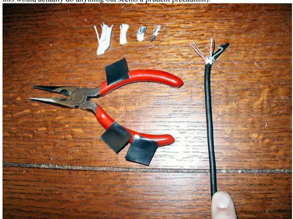
Step 4: Take you car charger and cut off the Palm adapter. Strip off a couple of inches of insulation exposing red and black (+) and (-) wires.
