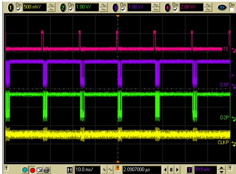
Figure 25: TE line trigger at 60Hz
