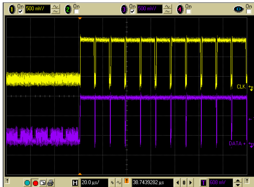
Figure 12: DDR_CLK_ALWAYS_ON = 0x0 and BLANKING_MODE = 0x0
